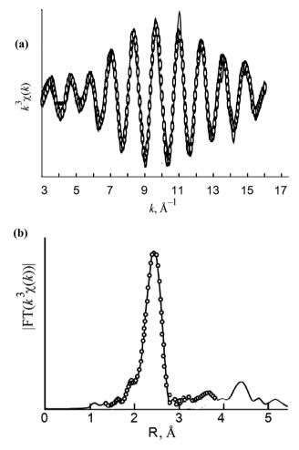
Fig. 3 (a) Experimental curve of normalized EXAFS signal (solid line) and optimized theoretical curve (points), and (b) modulus of the Fourier transform for the experimental EXAFS spectrum (solid) and its optimized theoretical curve (circle points) for the Tc<sub>x</sub>C sample with 50 at% C (parameters of local structure are given in Table 1).
