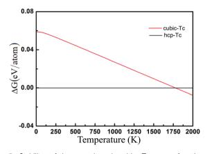
Fig. 5 Stability of hexagonal and cubic Tc as a function of temperature.
