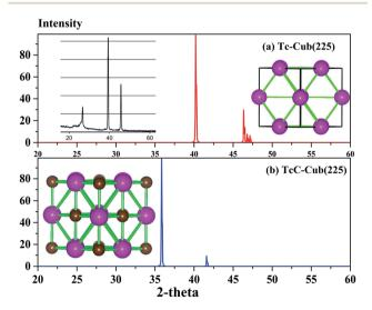
Fig. 4 In the inset in (a), we show the experimental XRD pattern of Tc metal and (b) NaCl-type TcC with the X-ray wavelength of 1.540562 Å. In (a), we illustrate the experimental XRD of Tc metal annealed with 50 at% C.<sup>25</sup>
