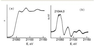
Fig. 2 XANES spectrum of (a) Tc K-egde, and (b) the first derivative for the Tc<sub>x</sub>C sample with 50 at% C.
