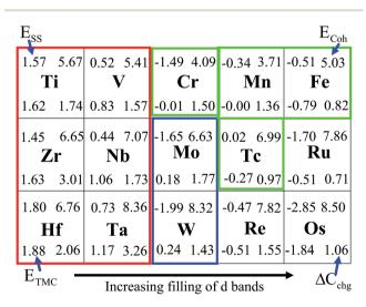
Fig. 1 Cohesive energies of TMs ( $E_{coh}$ ), C dissolution energies calculated using TM<sub>16</sub>C model ( $E_{C-dis}$ ), formation energies of TM monocarbides ( $E_{TMC}$ ), and charges captured by C atoms in TM monocarbides ( $\Delta C_{chg}$ ). NaCl- or WC-type TM monocarbides are selected in the light of  $E_{C-dis}$  values.
