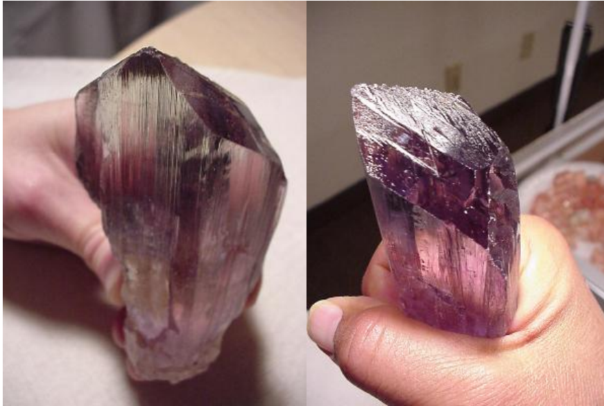
Demonstration of pleochroism of kunzite – its colour parallel to [001] is much stronger than in a perpendicular direction.
