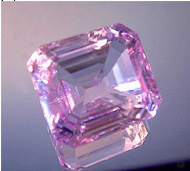
Cut kunzite. The colour is delightful, but unfortunately it gradually fades away when kunzite is exposed to daylight. It can be restored by radiation. This indicates that the colour of kunzite is due to point defects and the associated electronic centres in its structure. Another interesting feature: irradiated by UV- or visible light, kunzite absorbs the energy and then radiates it back – creating impressive glowing effect in the dark! Such a glowing effect is called luminescence when its duration is long, or fluorescence if its duration is short.
