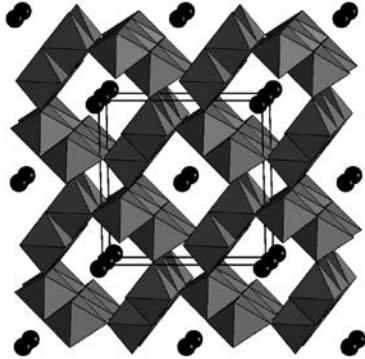
Structure of hollandite, showing Mn-centred octahedra.
