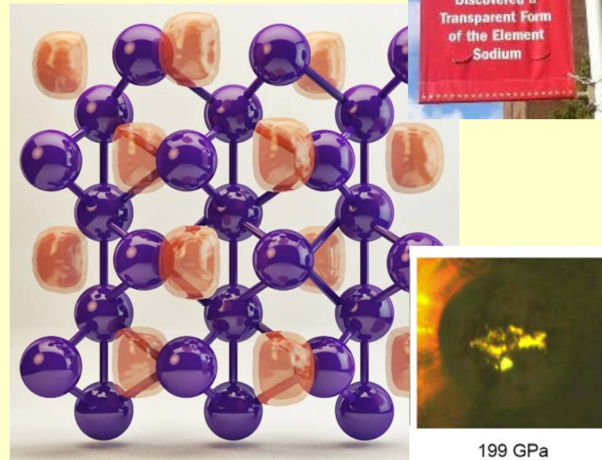
High-pressure transparent allotrope of sodium (Ma, Eremets, Oganov, Nature , 2009)
